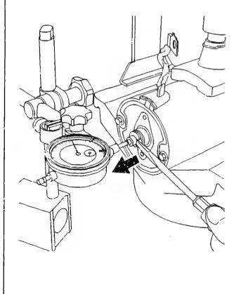
STARTING MOTOR ASSEMBLY Assembling bearing end plate Slip new gasket (1) onto commutator end shield. Fill 1/3 of bearing end plate (2) with grease and secure. Use torque wrench. Torque wrench: Grease VS 18036 Ft: comm. avail. 5 997 098 000
